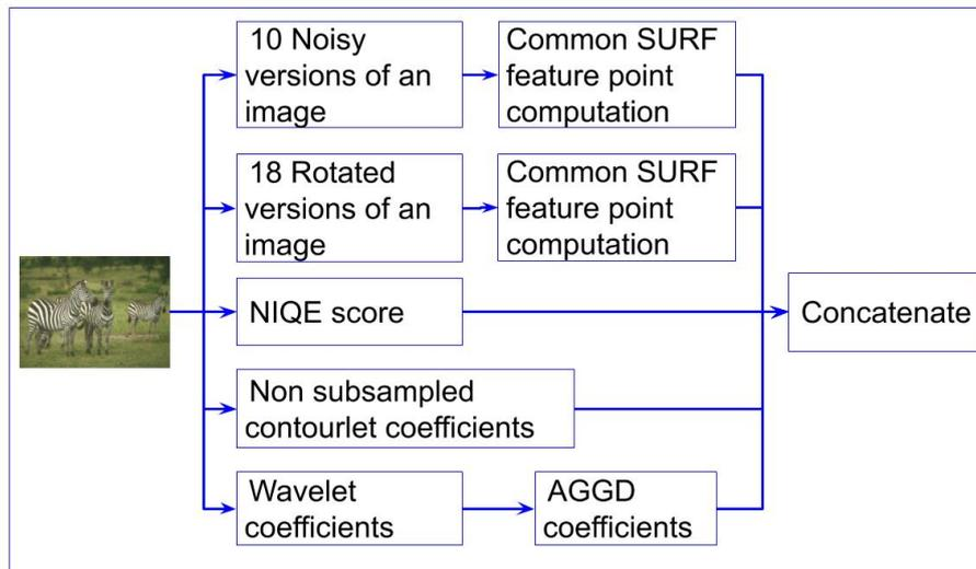
Figure 4: Feature extraction for GO-IQA. NIQE stands for Naturalness Image Quality Evaluator. AGGD - Asynchronous Generalized Gaussian Distribution, SURF - Speeded Up Robust Features
